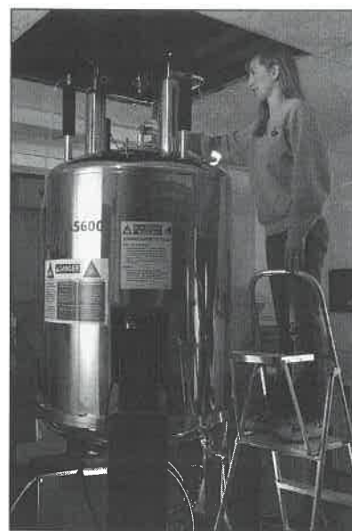
Loading a sample into the 600 MHz NMR.
