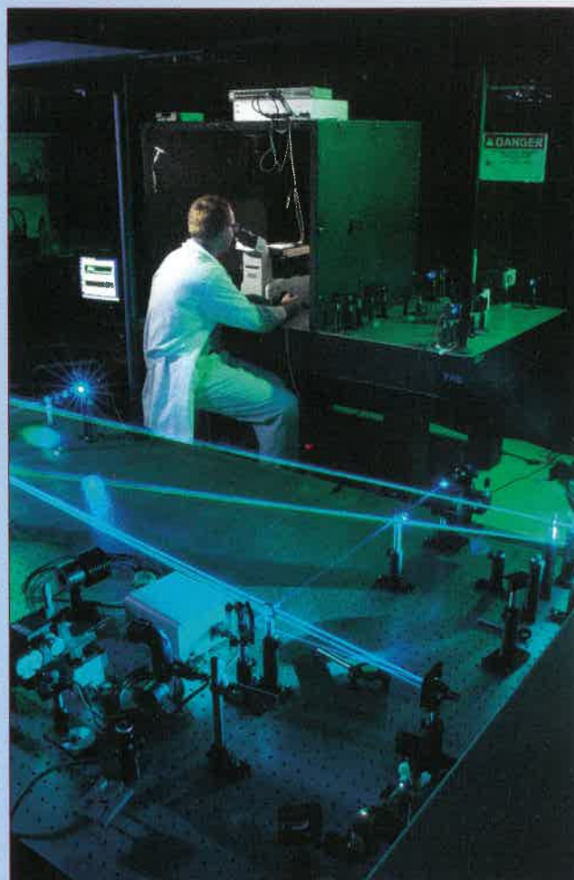
Single molecule fluorescence microscope system and laser source.
