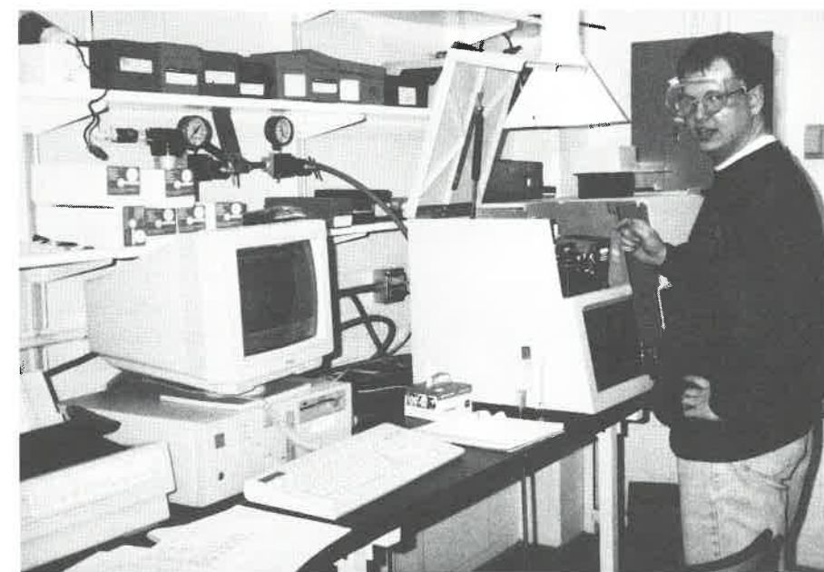
Undergraduate Rob Dufield works with an atomic absorption spectrophotometer in the new third floor instructional instrumentation laboratory.
